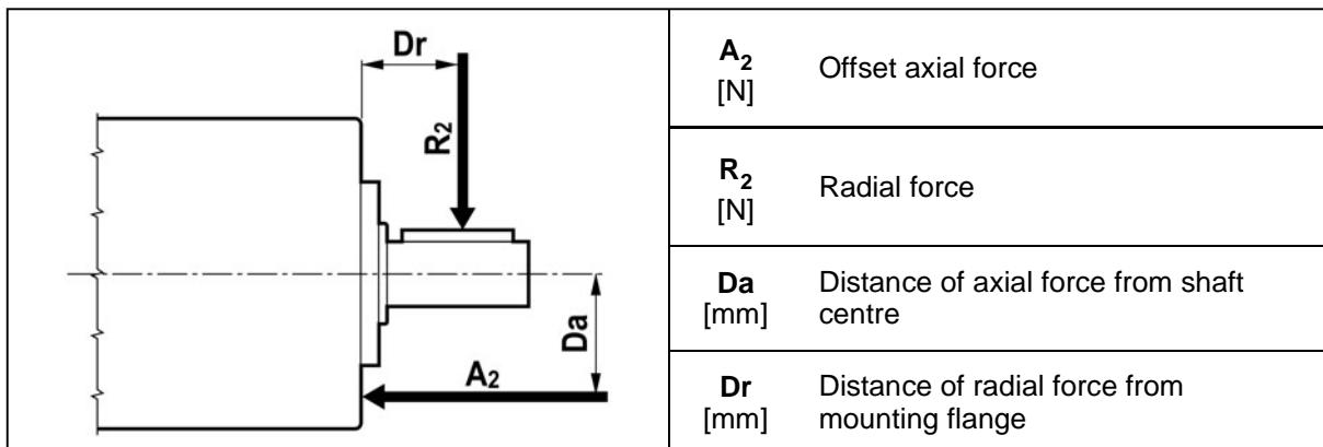
**SERVICE LIFE CALCULATION FOR RIGID BALL BEARINGS (CS)**
