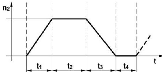
$$I [\%] = \frac{t_1 + t_2 + t_3}{t_1 + t_2 + t_3 + t_4}$$
